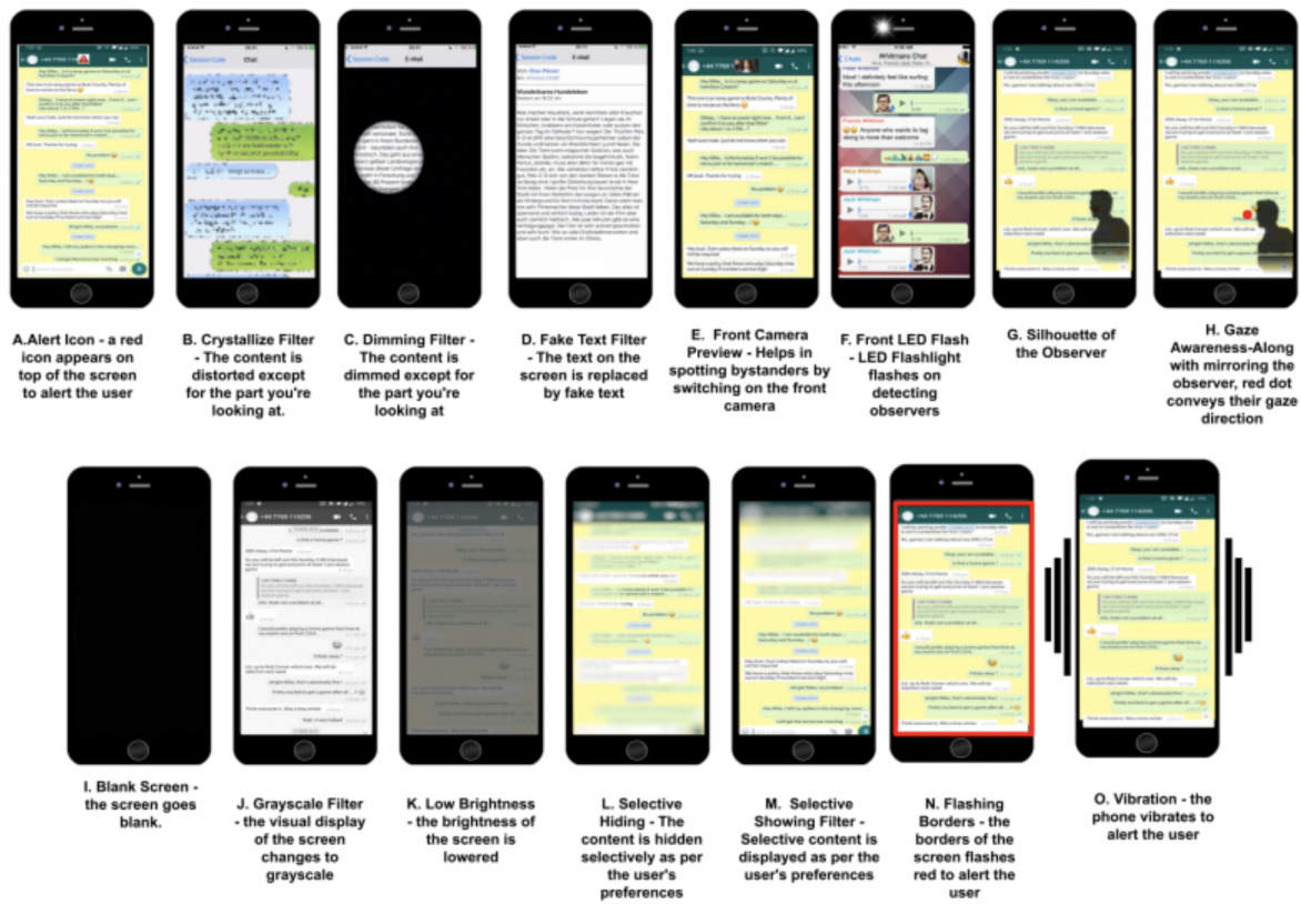
Figure 5: Presented Mechanisms to choose from that either alert the user giving the choice to the user to decide if he wants to have protect the view or mitigating the shoulder surfed content by applying an overlay or a filter
